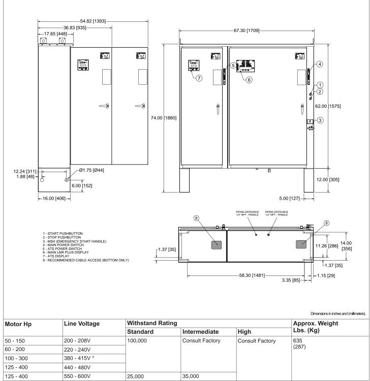
\* Coils Available: 380V-50Hz, 380V-60Hz, 415V-50Hz, 415V-60Hz
